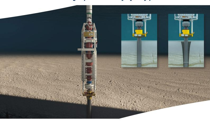
4Subsea's conductor analysis documents that the conductor can maintain required integrity during the entire lifespan of the well. By tailoring the analysis to the specific rig choice, well location and design, we reduce cost by maximizing the operational window and avoid oversized equipment.
