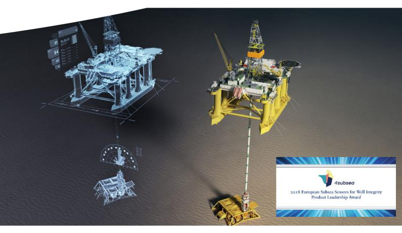
Subsea Wellhead Integrity Monitoring (SWIM<sup>™</sup>) measures accumulated load and other critical parameters on the wellhead during drilling operations, providing KPIs and prediction analysis as a digital service. No extra personnel are required on the rig.
