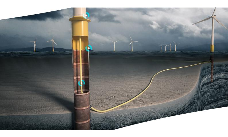
SMS Guard™ is a retrofittable instrumentation solution for monitoring of offshore wind turbine substructures. The magnetic sensors, combined with advanced machine learning algorithms and 4Subsea domain expertise, help operators realise the significant potential of reduced LCOE (Levelized Cost of Energy) using digital tools.
