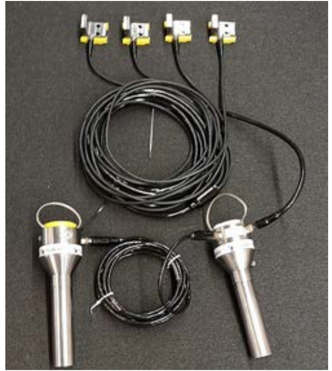
SMS Strain™ kit prepared for installation on BOP
